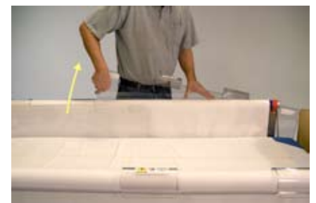
To remove the side rails take hold of the side and pull upwards.
