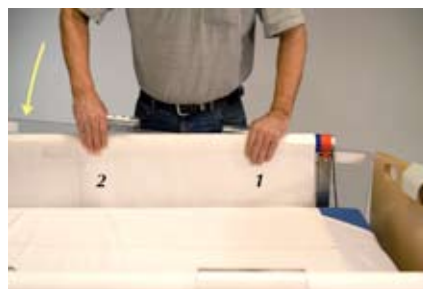
The easiest way to attach the side rails is to press the bent edges on to the bars one at a time.
